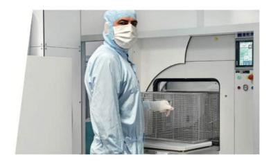
In the cleanroom production areas of TRUMPF Laser SE in Schramberg, strict cleanliness requirements apply. The MAFAC PALMA ensures the necessary particle and film cleanliness of laser components to maintain their full functionality. Particularly, laser-guiding components must be entirely residue-free to guarantee precise performance.
